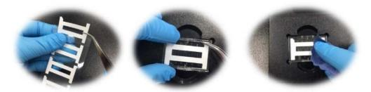
6 Place one end of sealing tape alongside left end of the test chip and seal entire holes. Then, scrub the surface of sealed points using finger, tweezers or scrubbing cloth enclosed in the package of GENECHECKER® UF-300 real-time PCR system.
