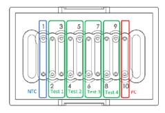
The 20µl of reaction mixtures prepared in 2.1 above is dispensed into two wells of the test chip corresponding to each target, with 10µl reaction volume. Well number 2 through 9 are used for detecting target genes while well number 1 and 10 are used for controls. Configuration of each well of the test chip is as following table.
