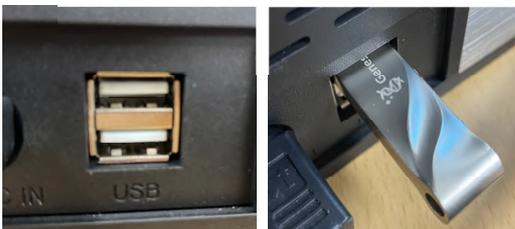
You can connect the external storage device to one of the USB ports located on the back of the instrument for transferring data files. Once storage device is connected, touch “Refresh” button to display up-to-date data file information.
